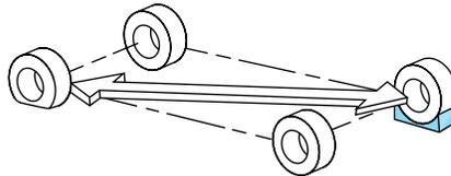
2. Turn engine OFF and block the diagonally opposite wheel (block not provided).
