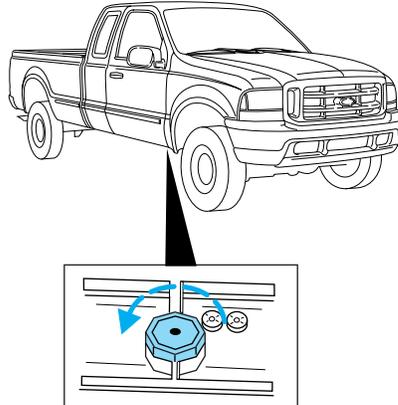
3. Fluid level should be at bottom of the opening.
