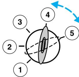
2. If the temperature is above  $-12^{\circ}\text{C}$  ( $10^{\circ}\text{F}$ ) and the engine does not start within five seconds on the first try, turn the key to OFF, wait ten seconds and try again.
