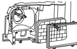
To install the new headlamp, reverse the removal procedure.
