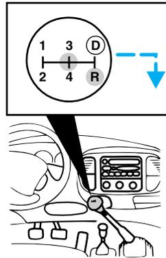
With the 6-speed transmission you can shift into R (Reverse) by moving the gearshift left from N (Neutral).
